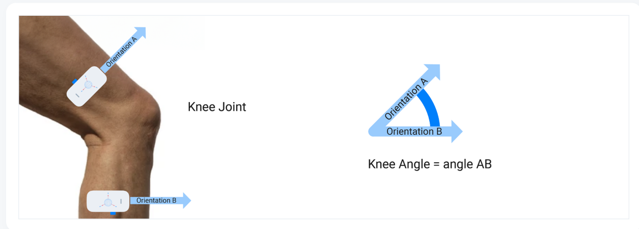
Figure 1.1. An illustration of how to use two IMUs to measure motion of the knee joint. In this image, only the sagittal plane is illustrated.
